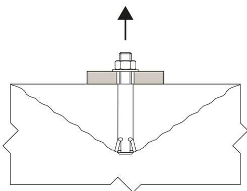
The realistic anchor behaviour is determined through centric tension tests
