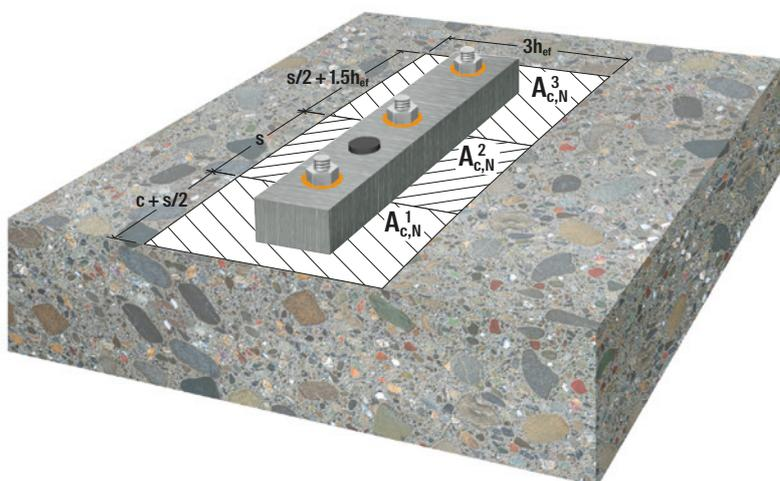
The tributary area approach is applied to individual anchors of a group in the framework of the non-linear spring model. The further modification factors as per the CC method are not required.
