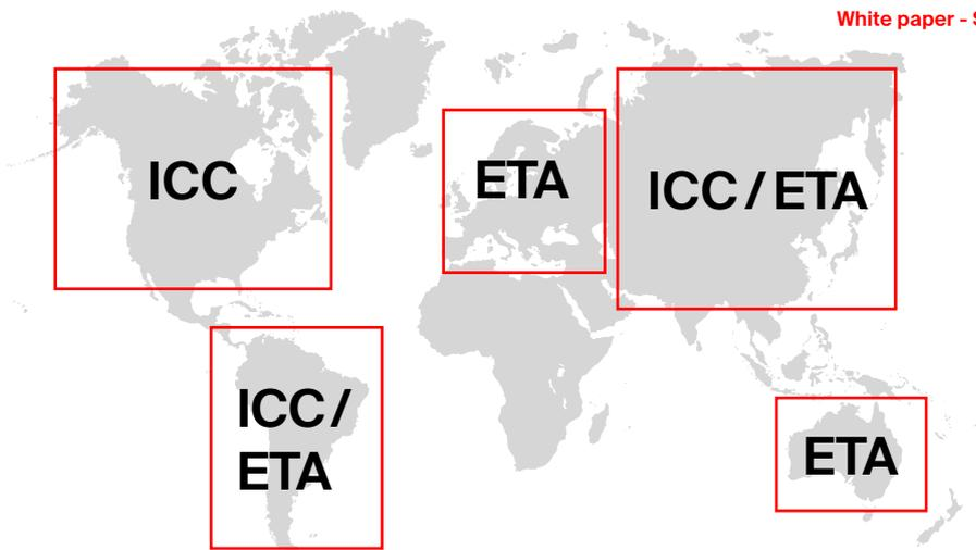
An overview of the prevalence of ETA (EN 1992-4) and ICC (ACI 318), the internationally recognised verification and qualification methods for anchorages in concrete.
