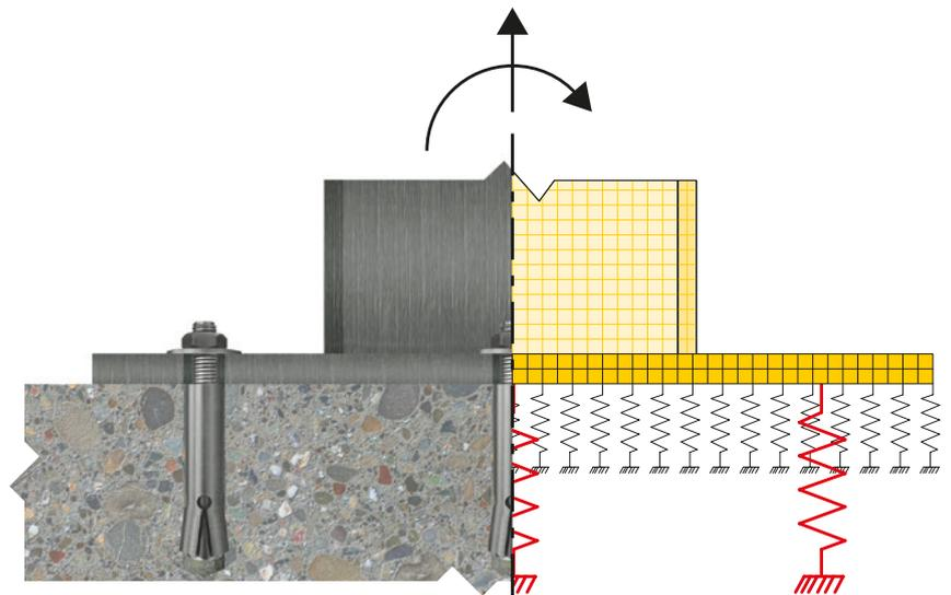
The purpose of an FE model is to subdivide a system into many smaller parts of finite size (finite elements). In this example, the base plate and the connecting profile are modeled using finite elements, the anchor springs and contact springs are modeled and the system is solved through FE calculation.
