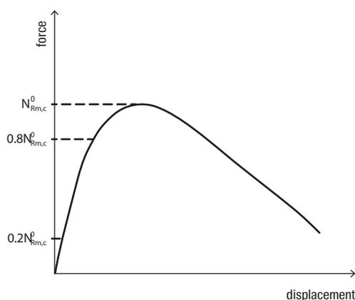
A load-displacement curve is obtained as a result of a tension test on the anchor
