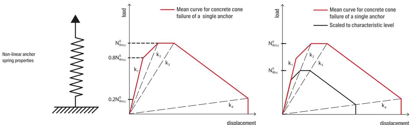
The load-displacement curve of a single anchor is idealised with a pentalinear format.
