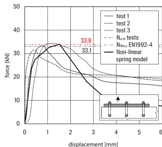
The non-linear spring model was verified through numerous tests on anchor groups in concrete (see PhD thesis of B. Bokor at the University of Stuttgart).
